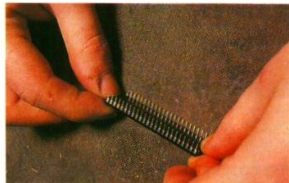
How to rectify it without pliers! Find a flat surface, and gradually bend the pin back into position. Actually a pair of pliers massively simplifies the operation, but steady, firm pressure is the basic requirement.
